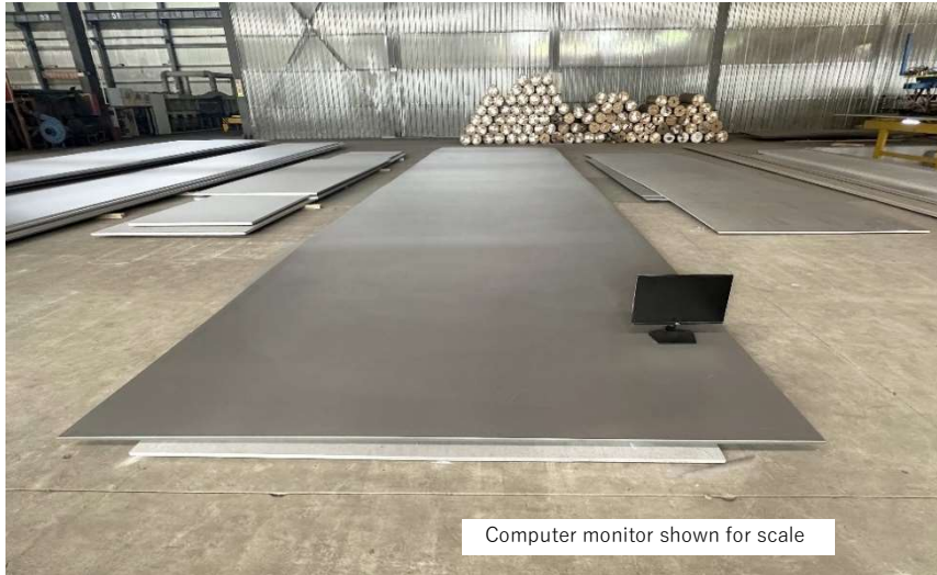
NAS625 ultrawide plate, 15 mm in thick and 3100 mm wide
