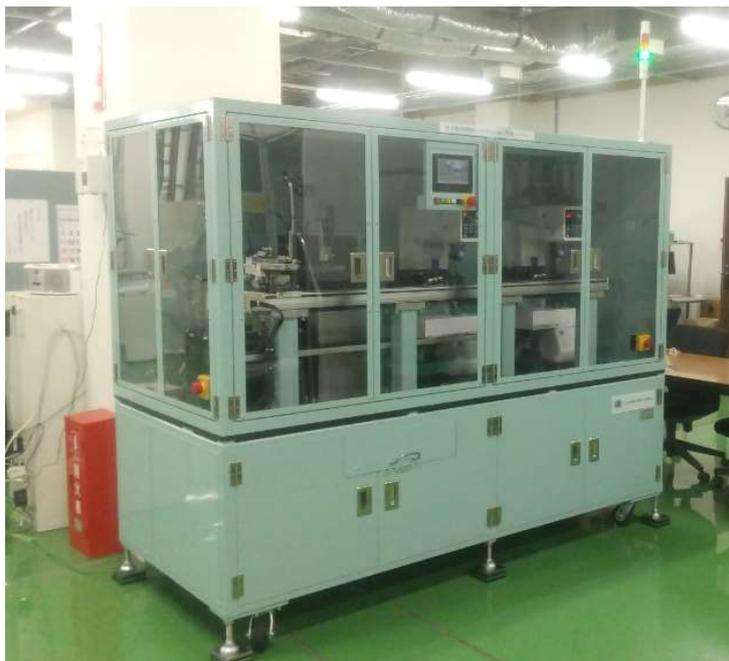
Automatic Rockwell hardness testing machine (For safety, it is enclosed with a steel frame and glass doors.)
