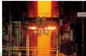
Continuous casting machine
