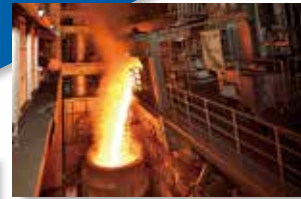
New electric arc furnace ("E furnace")
