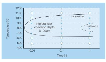
Test conditions: ASTM G28 Method A Test time 24h,
