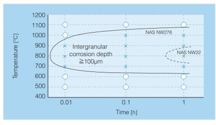
Test conditions: ASTM G28 Method A
