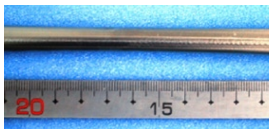
30% tensile test of NAS H840 plasma welded pipe
