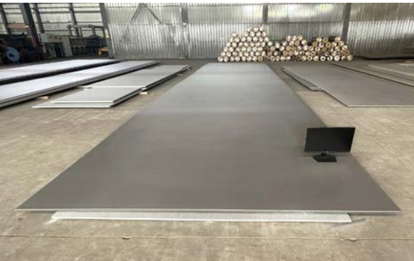
Ultra-wide nickel alloy plate 625 (15 mm thick x 3,100 mm wide) (monitor included as a size reference)
