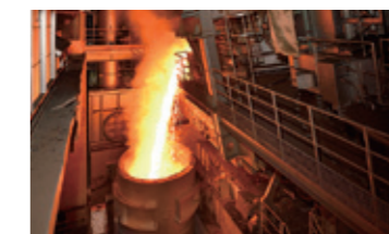
New electric arc furnace ("E furnace")
