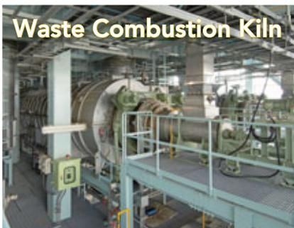
Measures are being undertaken to reuse waste that contains carbon and hydrogen in electrical generation plants by using the gas derived by carbonizing and gasifying the waste. NAS 800H, which excels in heat resistance, is being used in the body of such waste combustion kilns.
